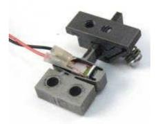
Figure 12 Extracted motor, without sensor magnetic scale
